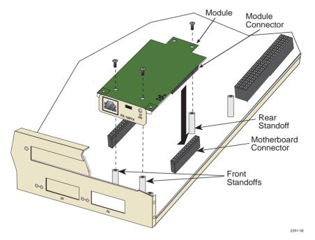
Figure C-5 Installing the Fast Ethernet Interface Module
